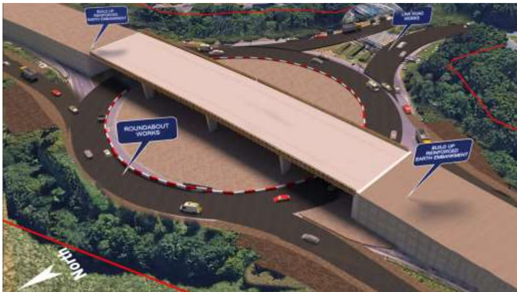
Figure 2 - Proposed Temporary Traffic Layout at South Terminal Roundabout During Reinforced Embankment Construction
